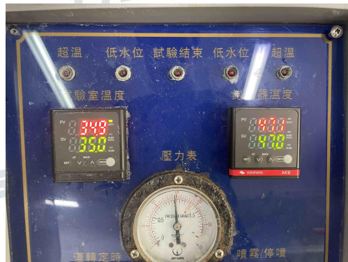
Salt Spray Test
